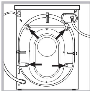
3. Remove the 4 protective screws and the rubber washer with the respective spacer, situated on the rear of the appliance (see figure).
