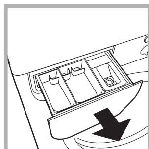
Remove the dispenser by pulling it out (see figure). Wash it under running water; this operation should be repeated frequently.
