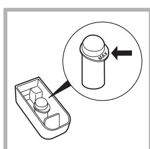
Place extra compartment 4, provided, into compartment 1. When pouring in the bleach, be careful not to exceed the "max" level indicated on the central pivot (see figure).
